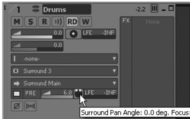
Figure 14.13 The Small Surround Panner is displayed on an aux send that is routed to a surround bus.
