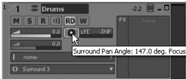
Figure 14.12 The normal Pan parameter of an audio track transforms into the Micro Surround Panner.
