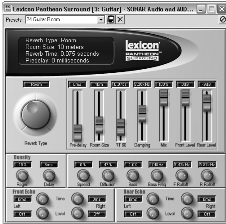
Figure 14.21 The Lexicon Pantheon Surround Reverb provides additional parameters for controlling reverberation in a surround environment.
