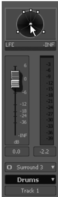
Figure 14.14 The Medium Surround Panner is displayed in the Track and Console views.
